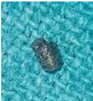
Figure 3: Retrieved abutment screw.
