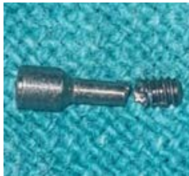
Figure 4: Fractured part with its upper part.
